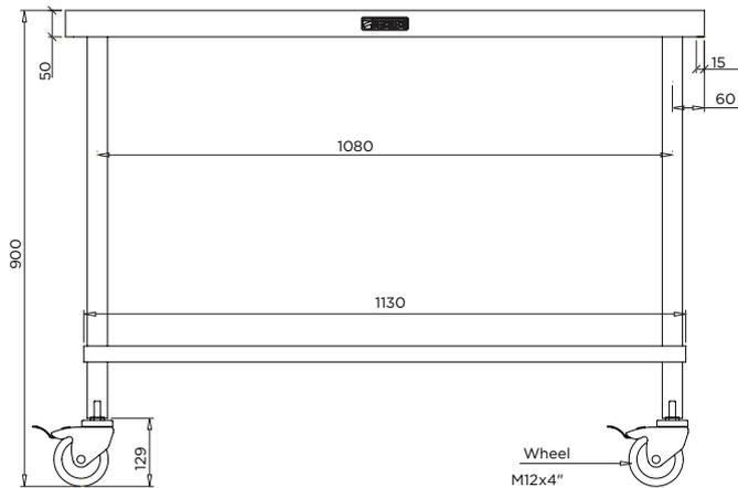
MODEL BT-MB-612 Front Elevation
