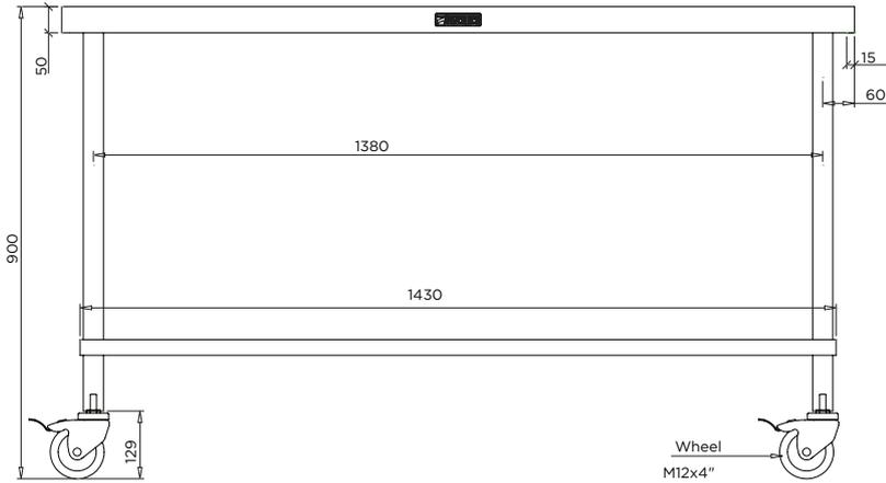
MODEL BT-MB-615 Front Elevation
